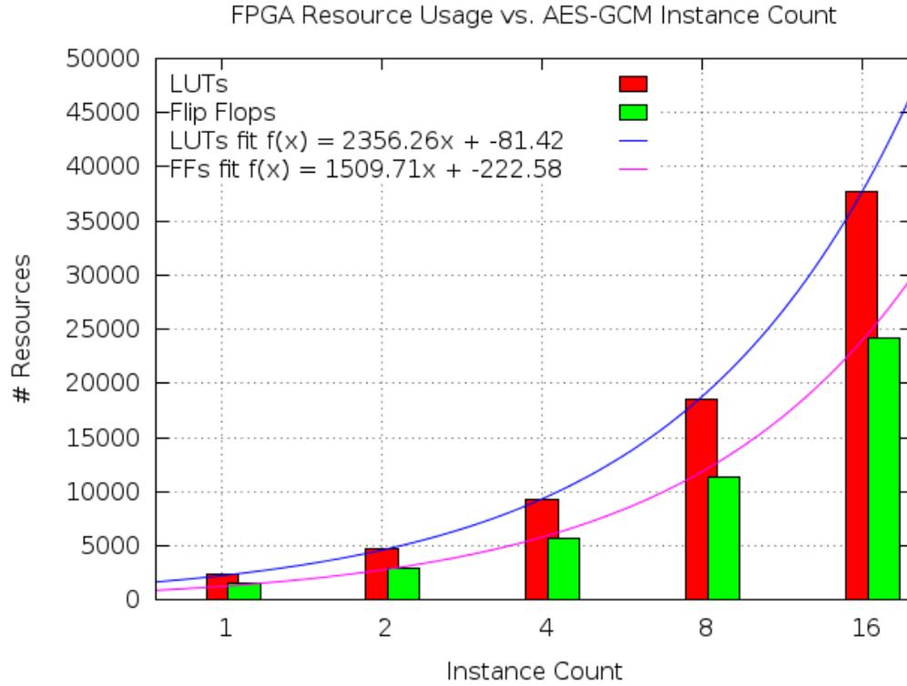
Figure 5.3: FPGA Resource Consumption for AES-GCM Modules
