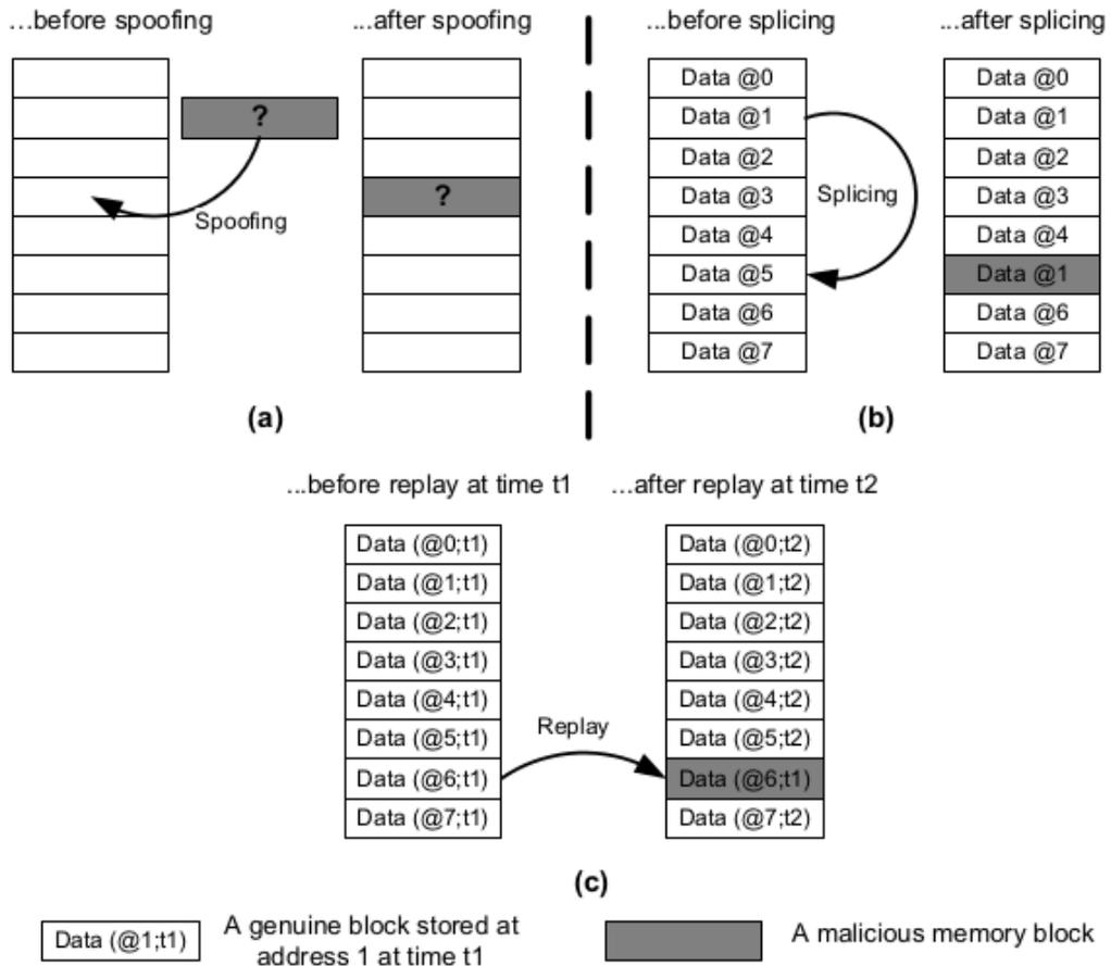
Figure 1.1: Spoofing (a), Splicing (b), Replay (c) Attacks on Memory (Adapted from Elbaz et al. [2])
