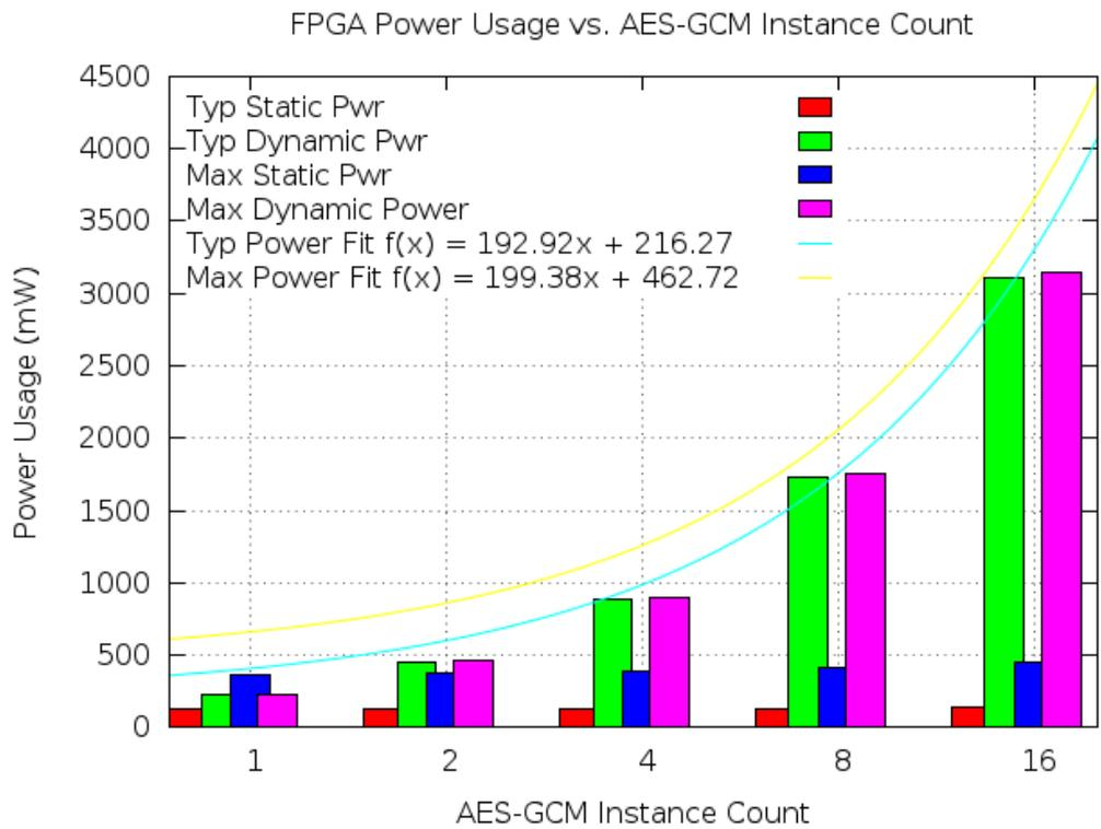
Figure 5.1: FPGA Power Consumption Estimates for AES-GCM Modules
