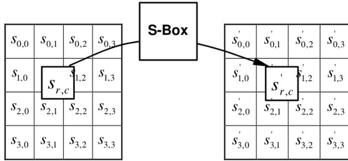
Figure 3.2: SubBytes Operation of AES (Image NIST [10])
