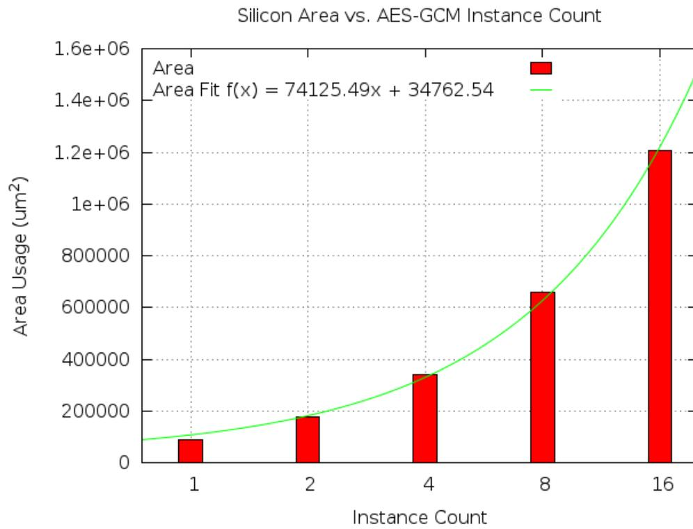
Figure 5.4: ASIC Area for AES-GCM Modules
