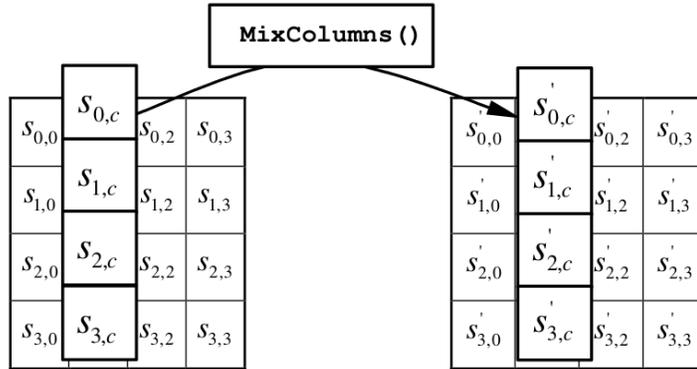
Figure 3.5: MixColumns Operation of AES (State Transformation) (Image NIST [10])
