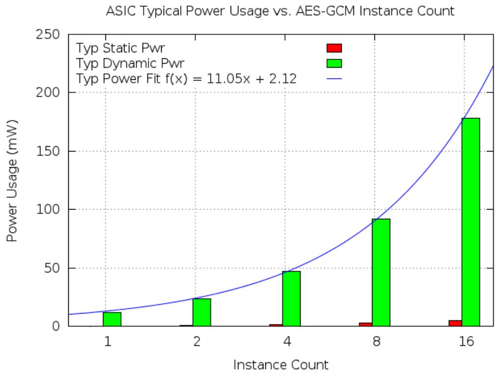
Figure 5.2: ASIC Power Consumption Estimates for AES-GCM Modules
