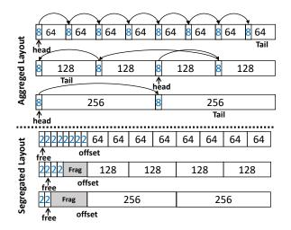
Figure 2: Metadata (pointers to blocks) shown in blue is decoupled from the allocated data in segregated layout whereas interspersed with data in aggregated layout. Data blocks are 64, 128, or 256 bytes.
